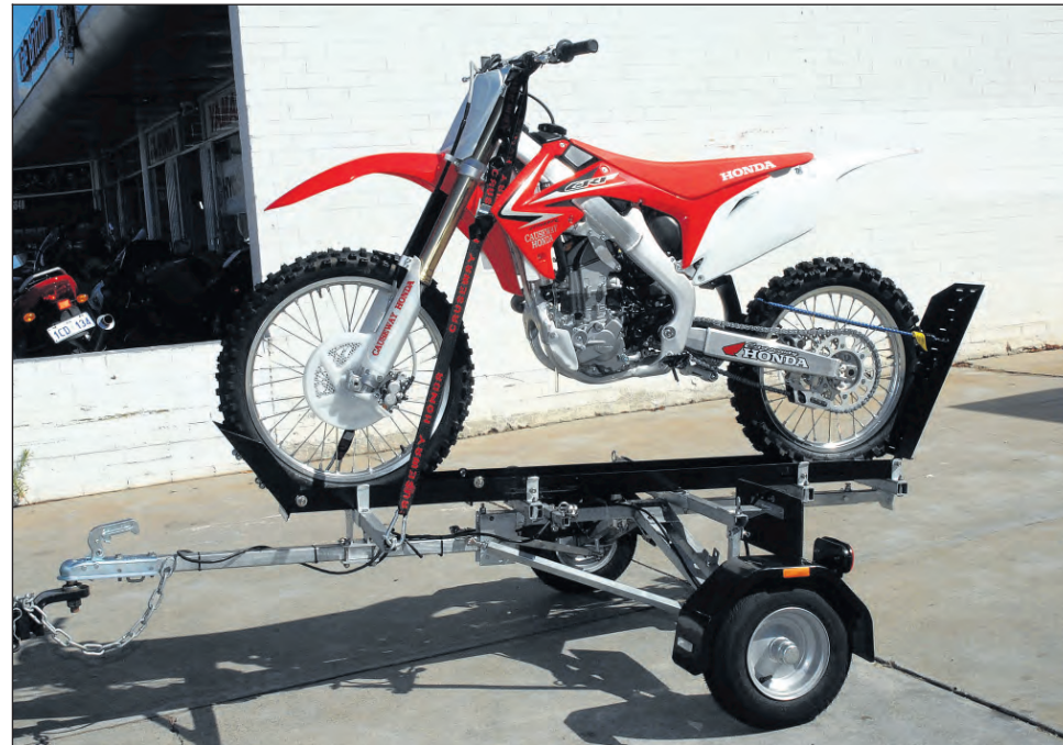
Ready to go: The trailer with a motocross, left, and in its folded state, below.
